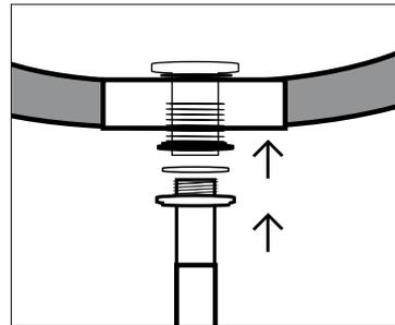
7. Thread the lock nut onto the threaded shank. Hand-tighten and make sure that the drain is properly aligned. When ready, finish tightening with a basin wrench to secure the drain.
