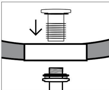
5. On the underside of the counter, attach the tapered rubber gasket. With the flat side facing down, slide the gasket up the threaded shank until it makes contact with the bottom of the sink.
