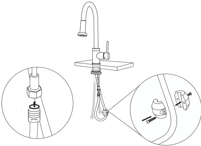
7. Once installation is complete, turn the main water supply back on from underneath your sink. Check for any leaks underneath.
