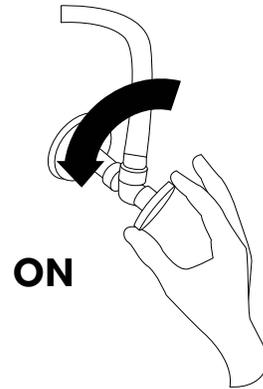
8. Remove the aerator from the faucet, and turn the faucet on for approximately 60 seconds to remove any dust or loose sediment within the water lines. Check for any leaks. Ensure that both hot and cold water are functioning properly. Reattach the sprayer nozzle and divert the water to the sprayer to ensure functionality.
