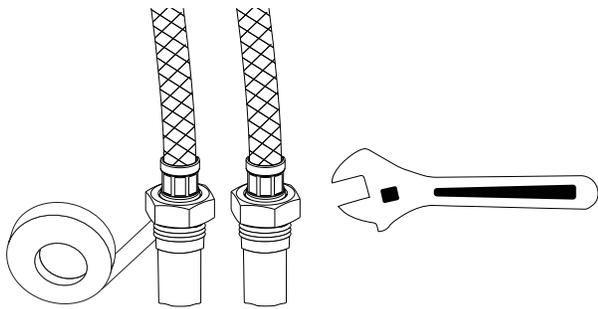
6. Insert the provided rubber O-ring into the hand sprayer's copper water line. Connect the hose for the hand sprayer to the copper line. Apply plumber's tape or thread sealant to the threads before tightening. Hand tighten the connections, then finish tightening with an adjustable wrench. Be very careful not to overtighten. Then, attach the provided weight to the nylon hose where the hose bends, as shown.
