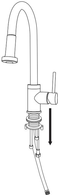
3. If not already attached, attach the provided braided water lines to the faucet. Apply plumber's tape or thread sealant to the threads before tightening. Hand tighten the connections, then finish tightening with an adjustable wrench. Be very careful not to overtighten.
