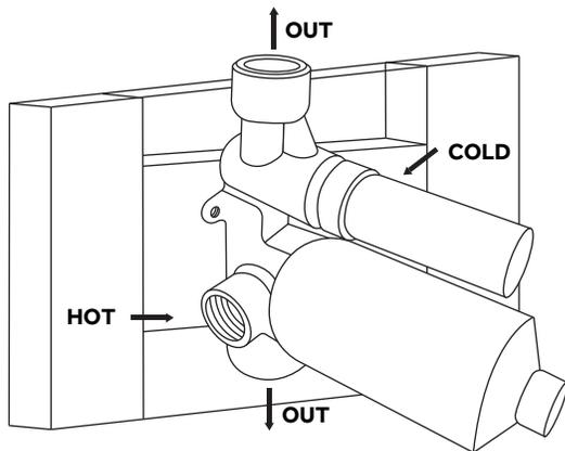
3. Route, assemble, and connect all in-wall piping to and from the shower valve. Make connections appropriately depending upon the type of pipe that is being used. For copper pipe, soldering will be required and should be completed by a licensed plumber. Apply plumber's tape to any threaded connections if applicable. Install any wood blocking that is necessary to support the piping and valve.
