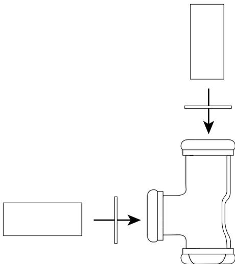
13. Attach the drain tube and flange to the waste and overflow tee with the sealing washer and slip nut. The beveled end of the sealing washer should face the tee.
