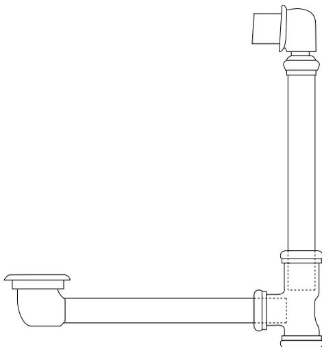
8. Remove the drain and overflow assembly from the tub, and trim the pipes at the marked locations with a hacksaw. Make sure that the blade is suitable for cutting metal.
