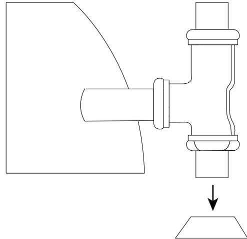
14. When your tub is in place and all connections have been made, fill the tub with water to check for any leaks from the connections. Verify that the drain and overflow is working properly.
