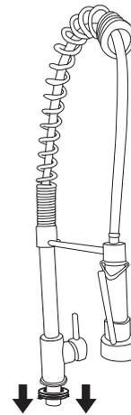
4. From beneath the sink, slide the rubber gasket back onto the faucet body followed by the metal washer. Thread the locknut back onto the faucet body using a basin wrench. Finish securing by tightening the two screws attached to the lock nut with a Phillip's screwdriver.
