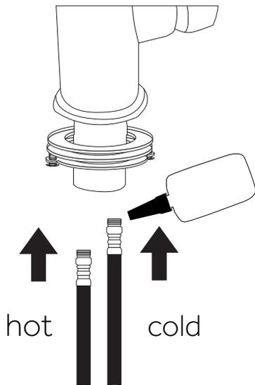
3. Remove the lock nut, metal washer, and rubber gasket from the faucet body. Insert the faucet body through the mounting hole in your counter top. Position the faucet so that the handle is on the left, as shown.
