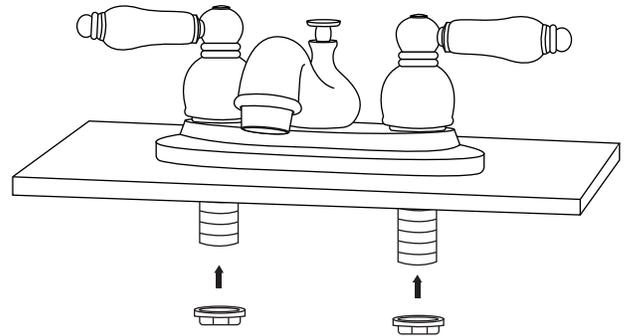
4. Connect the main water supply lines to the threaded shanks of the faucet. If needed, use the provided cone washers and lock nuts to make the connections. Apply thread sealant or plumber's tape to the threads before attaching.
