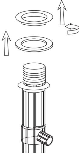
2. Set the flat rubber gasket over the drain hole in your sink, then insert the flange into the drain hole.
