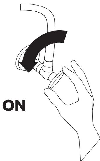
6. Remove the aerator from the spout and turn the faucet on to remove any dust or loose sediment from the water lines. Check for leaks. Check to ensure that both hot and cold water are running properly. Allow the water to flow for approximately 60 seconds, then reattach the aerator.
