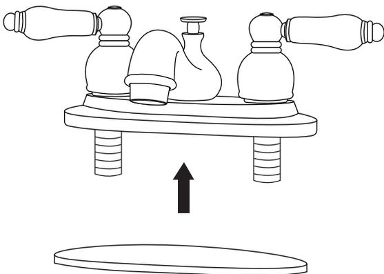
3. Insert the faucet into its prepared mounting holes. From below, secure the faucet by tightening the provided lock nuts onto each threaded shank. Hand tighten firmly. Finish tightening with an adjustable wrench if desired.
