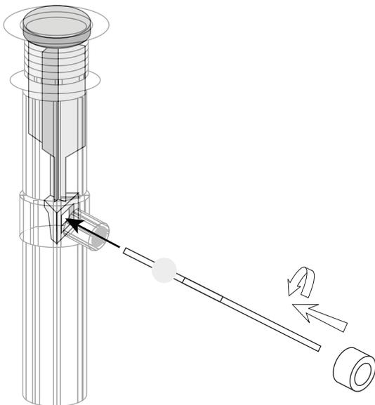
5. Position the drain so that the lever is facing the back of the fixture, in line with the faucet's lift rod. While holding in place, hand tighten the lock nut until secure then finish tightening with an adjustable wrench. Be careful not to overtighten, which can crack a fragile sink.
