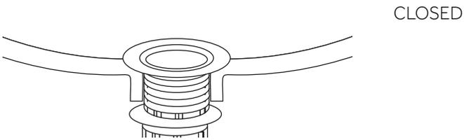
10. Fill your sink to check for any leaks and to ensure that the drain is functioning properly.
