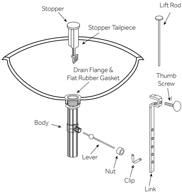
1. Remove the flange by unthreading it from the drain body. Remove the flat rubber gasket as well.
