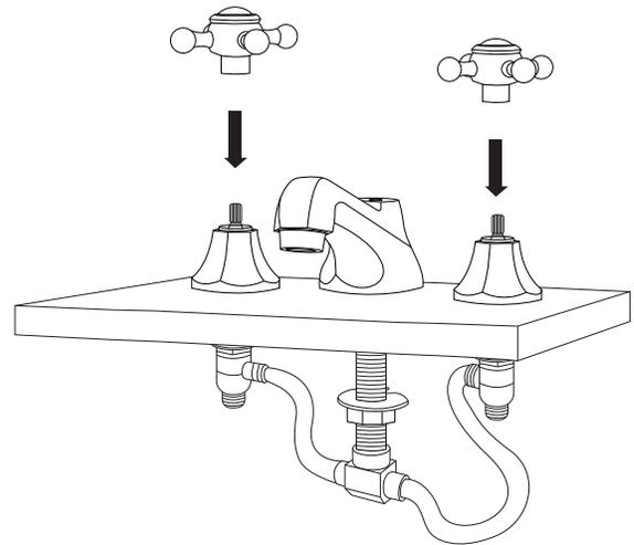
12. Connect the main water supply lines to the valve stems. Apply plumber's tape or thread sealant to the threads before tightening. Remove the aerator from the spout and turn the faucet on for approximately 60 seconds to allow any dust or loose sediment to exit the water lines. Check for any leaks. Test both hot and cold water to ensure they are running properly. Once testing is complete, reattach the aerator.
