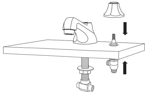
8. From beneath the sink, position the stem so that the outlet on the side of the stem is pointing inward, towards the T-connector. While holding in place, hand tighten the lock nut. Finish tightening using a basin wrench.
