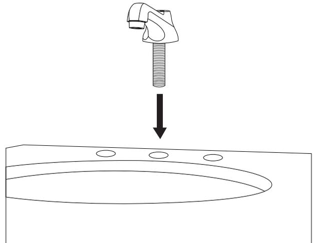
4. From beneath the countertop, slide the metal washer back onto the threaded shank. Hand tighten the lock nut, then finish tightening using an adjustable wrench.
