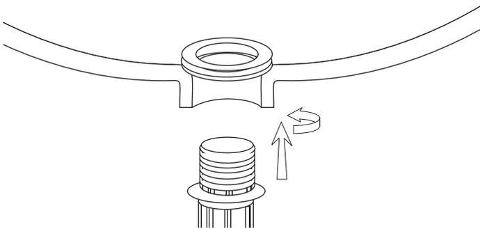
4. Connect the drain lever by threading it into the hole on the side of the drain body. The lever must pass through the hole in the stopper tailpiece to function properly. Apply a bit of thread sealant or plumber's tape to the threads before attaching.
