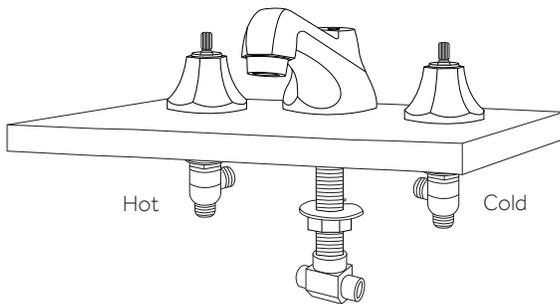
10. Use the provided braided water lines to connect the hot and cold valve stems to the T-connector. Use an adjustable wrench to tighten, but be careful not to overtighten. Apply thread sealant or plumber's tape to each threaded connection before attaching.
