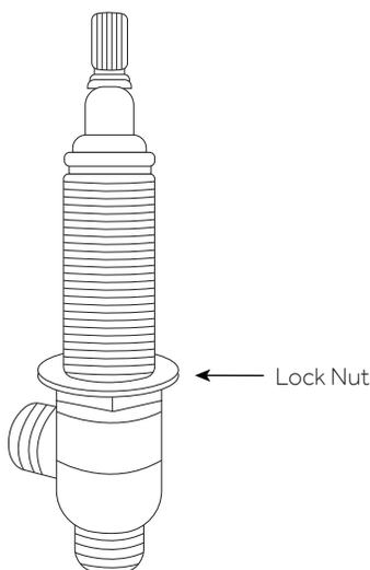
7. From beneath the counter top, insert the valve stem through the right-side faucet hole. From above the counter top, thread one of the two bell flanges to the stem until hand-tight.
