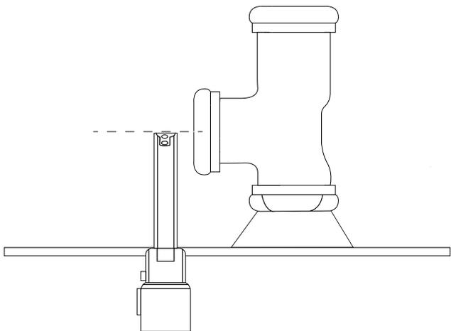
3. Carefully set the tub back into position and adjust the leveling feet as necessary. If your tub does not have leveling feet, shims may be used. Once level, apply a generous bead of silicone on the bottom of the feet. This will prevent the tub from shifting after installation.
