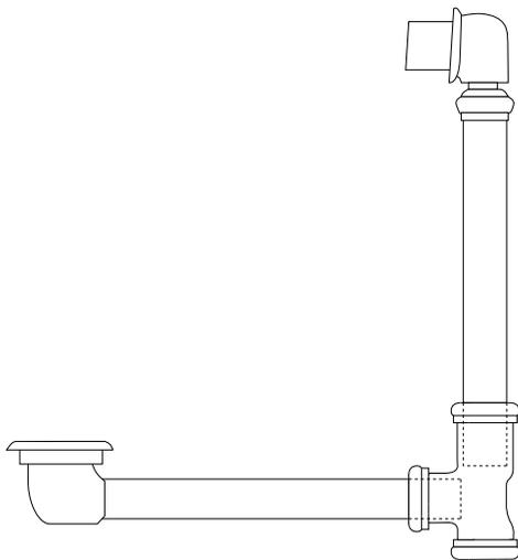
8. Remove the drain and overflow assembly from the tub, and trim the pipes at the marked locations with a hacksaw. Make sure that the blade is suitable for cutting metal.
