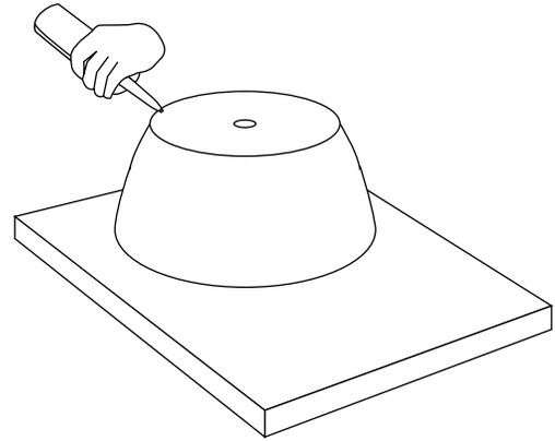
2. Turn the sink right-side-up and position over the 2" drain hole.
