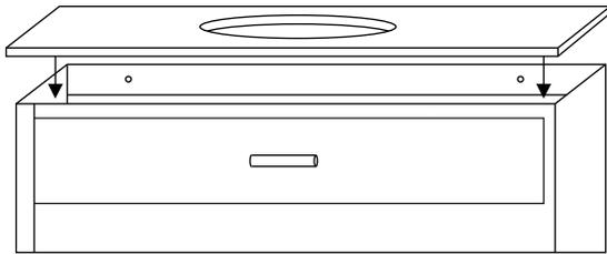
2. With assistance from another person, slowly and carefully set the countertop onto the vanity cabinet. Once positioned, press firmly into place. Wipe away any excess sealant using a damp cloth.
