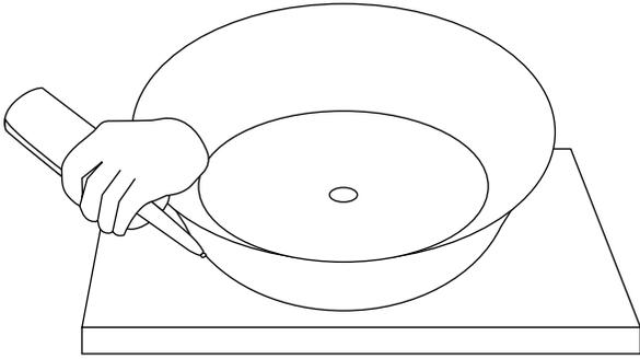
4. Remove any excess sealant to complete the sink installation.
