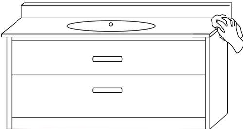
3. If you are installing a side-splash and/or back-splash, place a generous amount of silicone sealant on the back of it and press it into place against your bathroom wall. Fill any gaps that are left with silicone sealant. Wipe away any excess sealant with a damp cloth.
