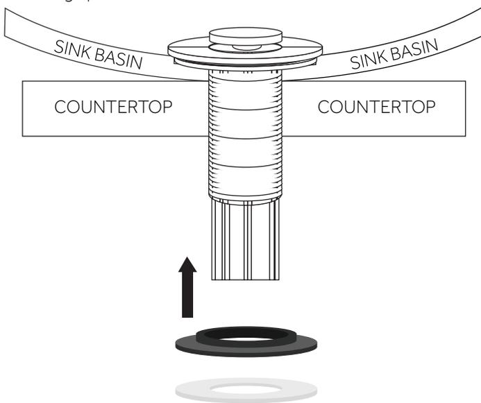
6. Thread the lock nut onto the drain flange. Hand tighten until secure, then finish tightening with a basin wrench once the drain is properly aligned.
