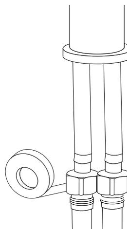
8. Turn on the main water supply. Remove the aerator from the spout and turn the faucet on to ensure that there are no leaks. Check to ensure that both hot and cold water are running properly. Allow the water to flow for approximately 60 seconds to remove any dust or sediment within the water lines. Turn the faucet off and reattach the aerator.
