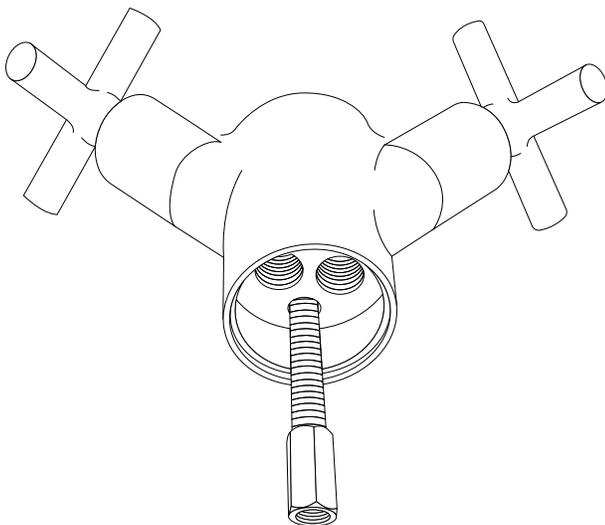
3. Apply plumber's tape or thread sealant to the threading on each braided water line, and attach them to the faucet body.
