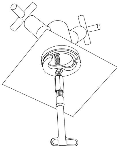
6. Insert the spout into the faucet body. Press the spout firmly into the body. Tighten the set screw on the back of the faucet body to secure.
