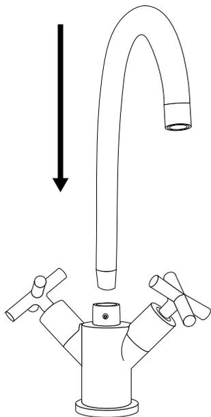
7. Attach the faucet's water lines to the main water supply. Apply plumber's tape or thread sealant to the threads before attaching. Tighten using an adjustable wrench, but be careful not to overtighten.
