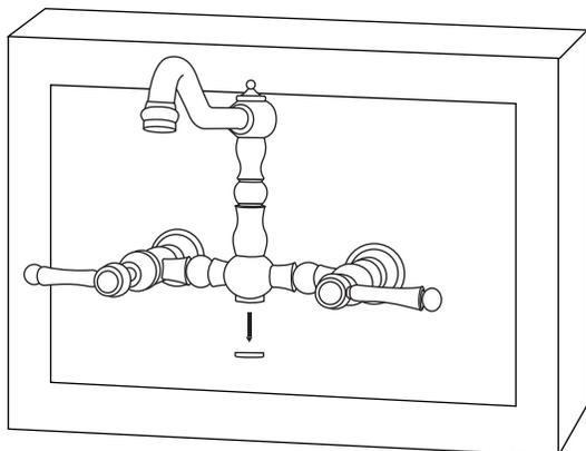
7. Once the plug is removed, attach the side spray hose to the outlet. Tighten firmly to ensure a water-tight seal.
