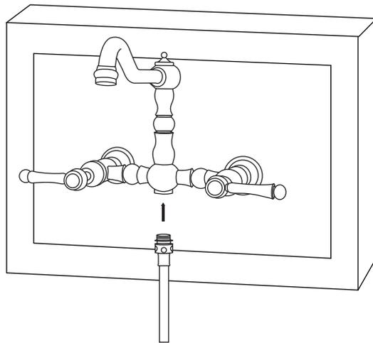
8. Attach the side spray to the opposite end of the side spray hose. Insert the provided rubber O-ring into the end of the hose before attaching. Hand tighten the connection firmly.
