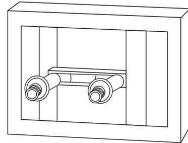
4. Insert one of the two provided screen washers into each of the installed couplers. Attach the faucet body by threading each handle base onto the installed couplers. Apply thread sealant or plumber's tape to the threads before attaching. Tighten firmly using an adjustable wrench.
