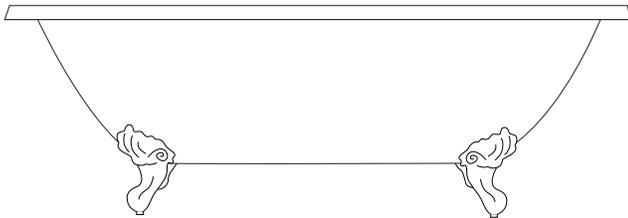
6. If the tub feet do not sit flush on the floor, shims may need to be added to the feet. To add shims, remove the foot and install the shim between the foot and the foot bolt. When the foot is aligned properly, secure it back to the tub.
