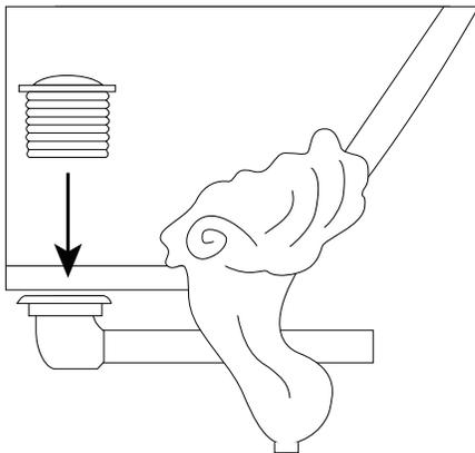
11. Install the overflow assembly with the beveled washer, overflow plate, mounting screw (provided) and any other washers or rubber sealing gaskets included.
