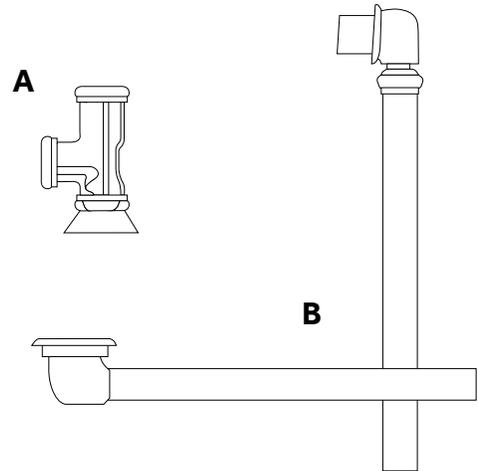
7. Measure and mark each pipe so that the end of the pipe reaches a little over halfway into the overflow tee.
