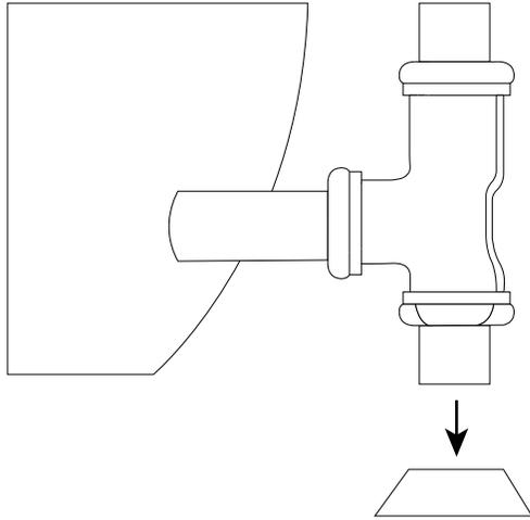
14. When your tub is in place and all connections have been made, fill the tub with water to check for any leaks from the connections. Verify that the drain and overflow are working properly.
