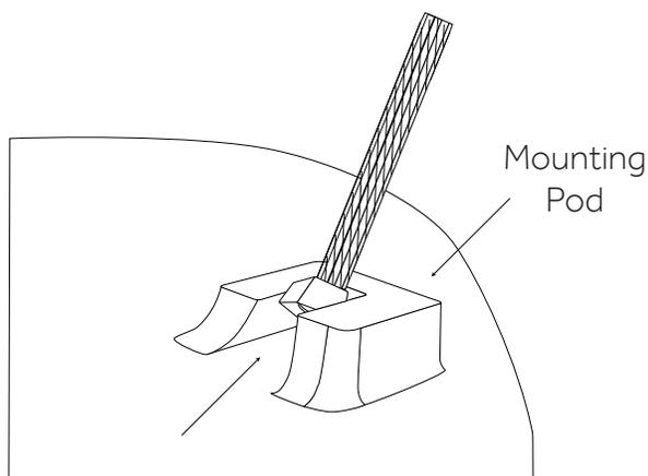
3. Match each tub foot with its corresponding pod, as shown below. If the letters on your tub and feet do not match, lay the feet out on the floor and check to see if all feet are the same size. If one pair of feet are slightly shorter than the second pair, then the shorter pair are meant to mount on the side of the tub containing the drain hole.
