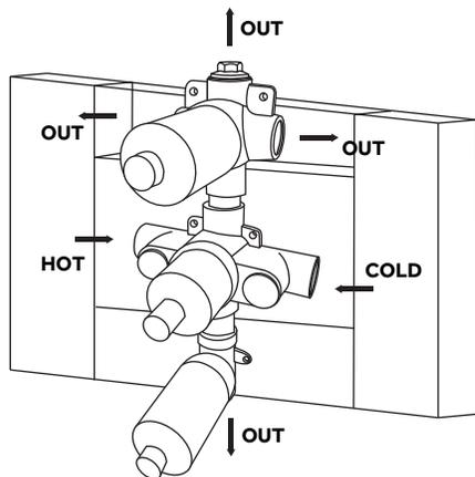
3. Route, assemble, and connect all in-wall piping as desired to and from the shower valve. Make all connections appropriately depending upon the type of pipe that is being used. For copper pipe, soldering will be required and should be completed by a licensed plumber. Apply plumber's tape to any threaded connections if applicable. Install any wood blocking that is necessary to support the piping and valve.
