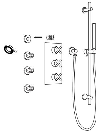
10. Attach the shower arms by threading each of them into their prepared female fittings. Be sure to use the decorative escutcheons to conceal the rough-ins. Apply thread sealant or plumber's tape to the threads before tightening.
