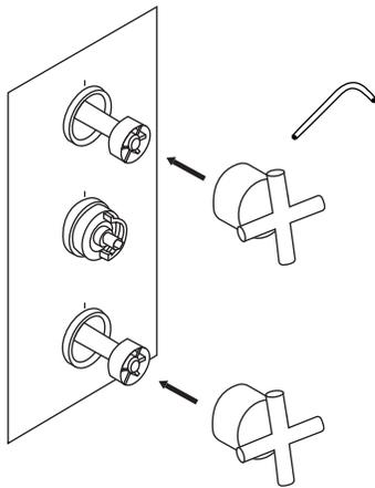
4. To install the temperature control handle, loosen the set screw and remove the handle from the handle base. Attach the handle base to the center stem using the provided screw. Tighten with a Phillip's screwdriver, then reattach the handle.
